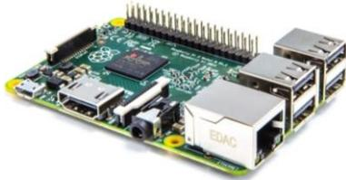
Gambar 3 Raspberry Pi 2 Model B
